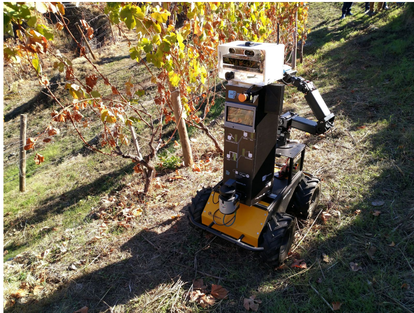
Figure 78: The AgRob V16 agriculture robot monitoring a slope vineyard.
