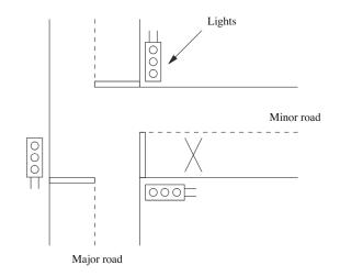
In this scenario vehicles drive on the left side of the road and the cross in the picture represents a sensor that tells whether a car is waiting in the minor road or not.
