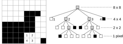
(Source: Wikipedia) shows how an image (in this case in black and white) is represented in the form of a quaternary tree (vulg. quadtree) by successive divisions of the 2D space into four regions, until reaching the resolution of one pixel.
