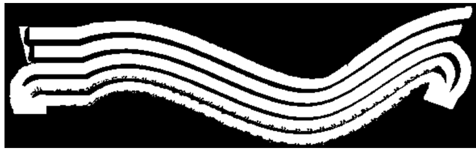
Figure 3. Occupancy grid map of a steep slope vineyard.
